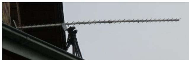
55 el yagi used to copy 23 cm EME beacon by DL6EDF
