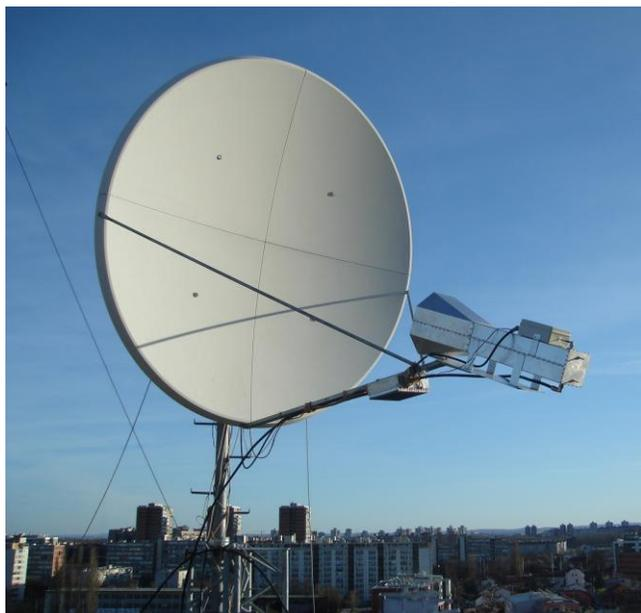
9A5AA's 2.4 m offset dish expanded to 3.5 m & septum feed with octagonal flare
