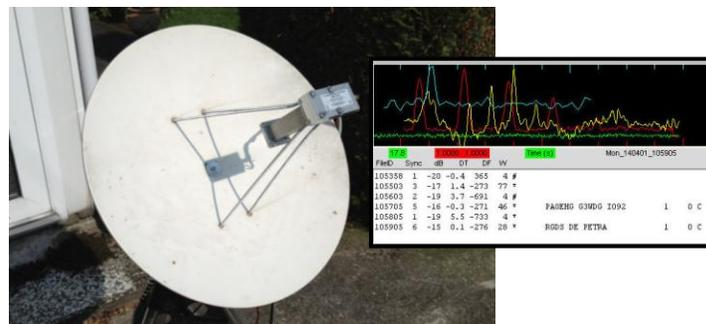
PA0EHG's 48 cm dish aimed to the sun and the signal from DL0SHF WSJT in high power (vertical scale 2 dB/div) and the carrier from G3WGD (vert scale 1dB/div) and decodes from G3WGD.
