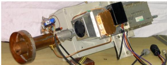
**The transverter is in the grey box. The feed is a SM6FHZ septum fed Kumar design. The whole thing is secured by 3 wing nuts and supplied through four plug connected leads for easy switching.**
