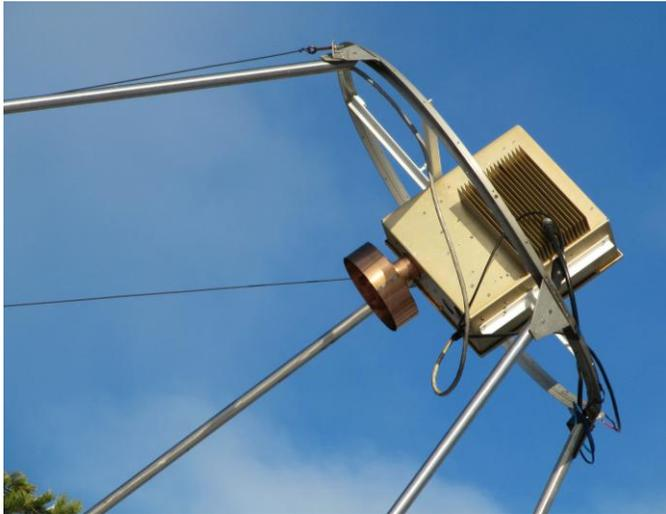
**OH2DG's 9 cm feed arrangement – includes RA3AQ feed, DB6NT transverter and 4 x Ionica 40 W SSPAs**
