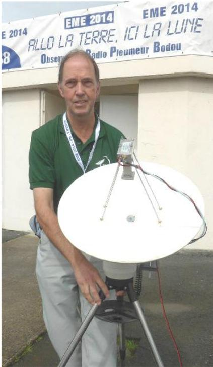
**PA0EHG with 0.5 m used to demo 10 GHz EME**
