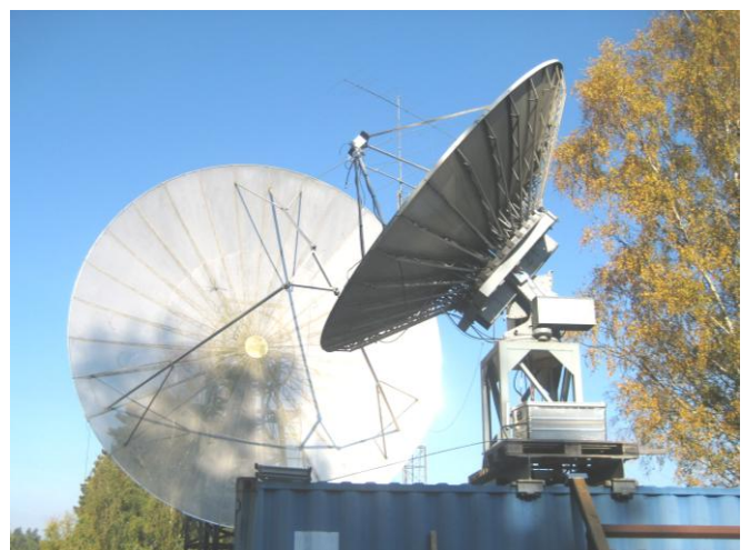
SM6CKU's new 4 m dish for MW EME with his old 8 m dish in the background
