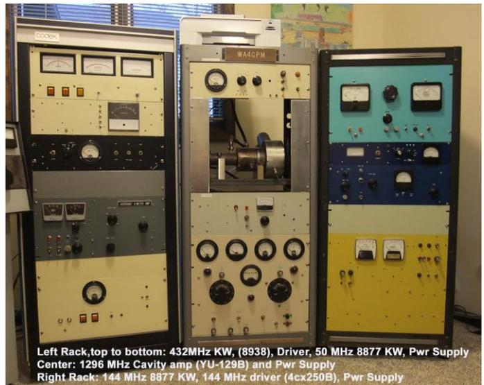
Left Rack, top to bottom: 432MHz KW, (8938), Driver, 50 MHz 8877 KW, Pwr Supply
