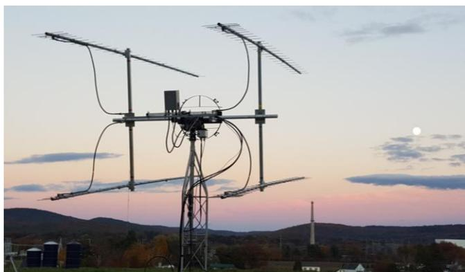
**N1VT 4 x FO25 yagis with 900 W at feed used on 432**
