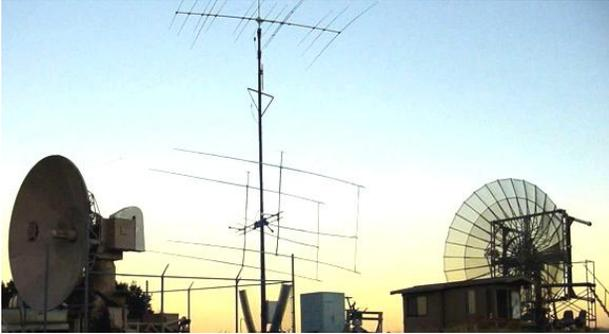
**W6YX site: 4.6 m 10 GHz dish (L), 2 m EME array (C), 8 m 13/23 cm dish (R)**
