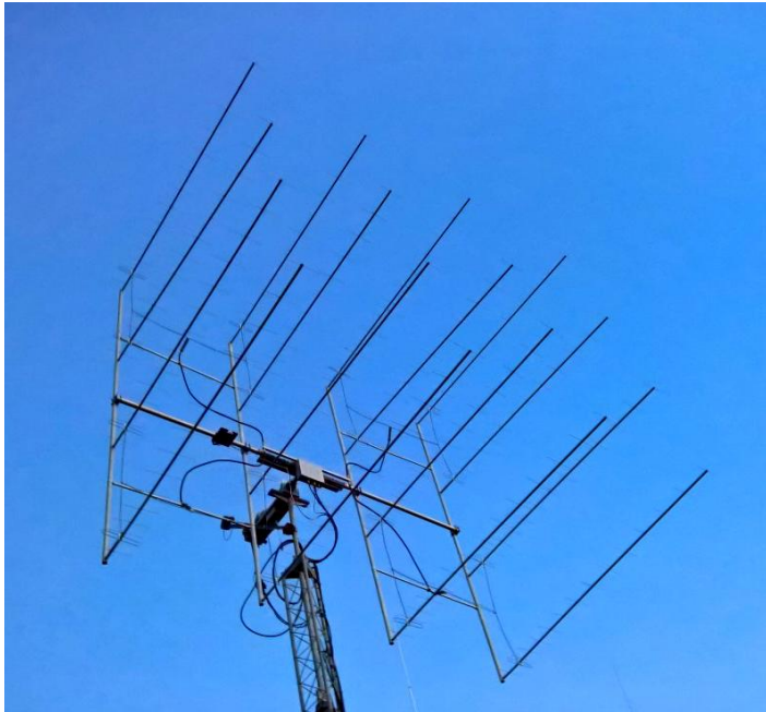
VK4EME's rebuilt array ((16 x 15 DL6WU yagis)
