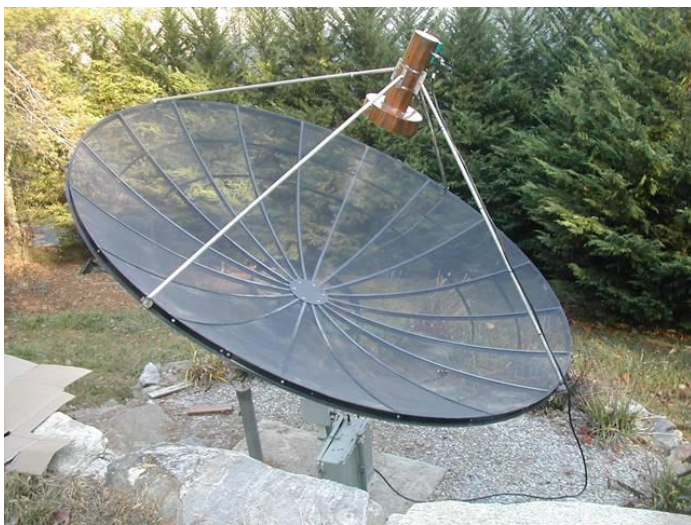
W4OP rebuilt 12' dish with 1296 feed
